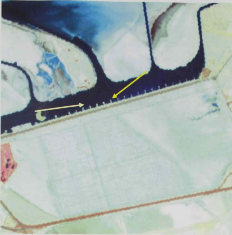
Figure 4-8: A close up Landsat-7 ETM image showing the sea breakers that appeared in the time for the period 1993-2000.
